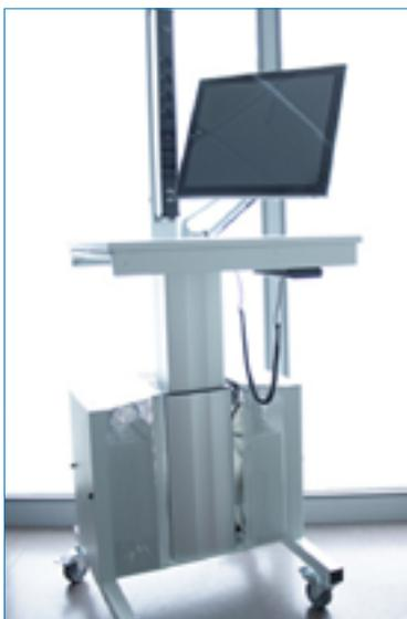
Our ‚device stations‘ are mobile docking stations for the measuring devices. All of them are equipped with a computer IT-certified for safety, a touch screen, a medical keyboard, a height-adjustable table and multiple sockets. All components are installed to a stable unit on wheels. We were able to realize the following optimizations by the development of the ‚device stations‘:
