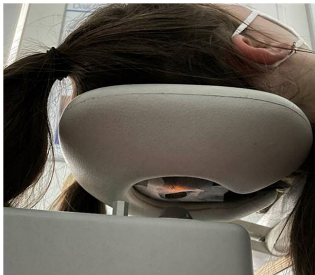
FIGURE 2 Placement of the subject's head on a specific head rest above the measurement window of the Raman device
